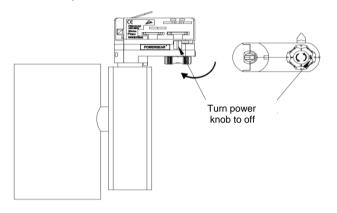
2. Make sure the track adapter flange is in the same track plane Then put the track adapter into the track
