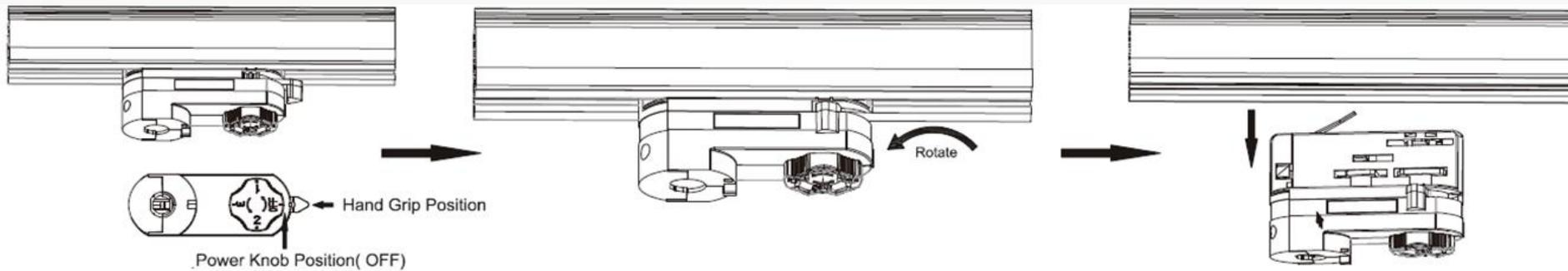
1. Make sure the track adaptor's positions are the same as the picture shows before removing.
